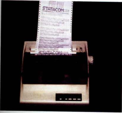
Figure 1.5 Dot matrix printers are impact printers – these are used to produce output on pre-printed forms, which may be single sheets or continuous forms
