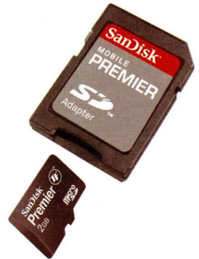
Figure 1.13 Miniaturisation is evident in memory card creation; over time, the physical card sizes have become smaller
